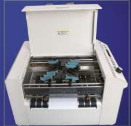
Eight HP 45 cartridges deliver high quality printing at blazing speed
